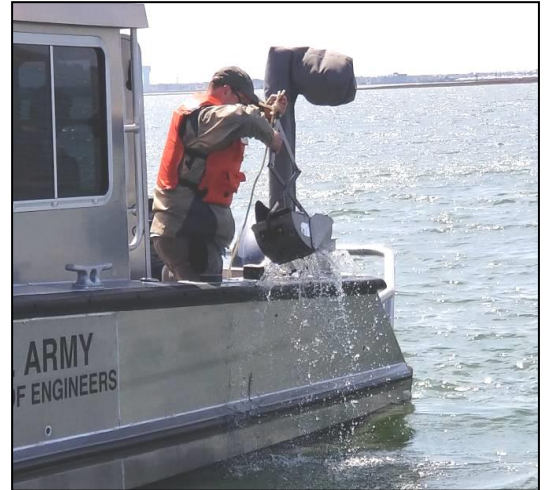
Above: USACE researcher takes a sediment sample from the NJ Intracoastal Waterway Channel
