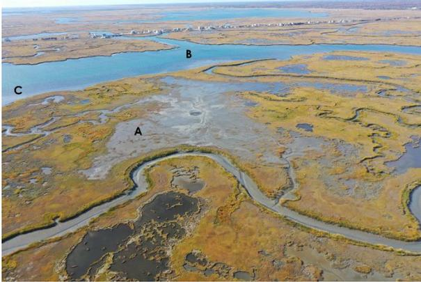
Figure 2 - Constructed marsh restoration (A), marsh edge protection (B), and intertidal shallows enhancement (C) with fine sand and mud at Gull Island (photo courtesy of Gary Paul, 2020).
