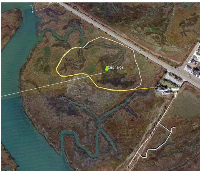
Left - Low lying marsh restoration area (white) showing potential location of biodegradable coir logs (yellow) to direct flows, and possible discharge point (green). Below – marsh conversion at the project site.
